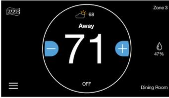
If you have an **EcoNet Zoning System** and the EcoNet Zone Control 'Away' heat set point is set to 50°F (10°C) or the cool set point is set to 92°F (33°C), the Zone Control will default to Off. Adjusting the 'Away' heat set point as low as 51°F (11°C) and the cool set point up to 91° (32°C) will allow the zone to be conditioned when required.
