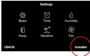
To enter the Installer Settings menu, select Menu > Settings, then tap and hold on "Installer" on the bottom right of the screen for five seconds.
