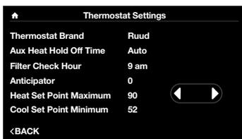
**Thermostat Brand** – The EcoNet Smart Thermostat will automatically populate when the system starts up by reading the equipment's model data card.
