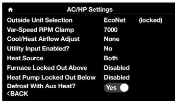
**Heat Pump Locked Out Below** – Selects the outside temperature below which the Heat Pump will not operate and your system will rely exclusively on the furnace or auxiliary heat source. This should be determined by evaluating the regions Heat Pump Balance point.
