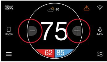
You can manually adjust the temperature from the Home Screen by touching the plus and minus buttons. When the set point is being changed, the ring will either turn blue or red—depending on the mode of operation—and the new set point is displayed in the center of the screen. If Auto mode is selected, press the lower left set point (red) for heat or lower right set point (blue) for cool.
