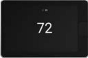
The standby screen can be turned off by disabling the back-light under basic settings (Menu > Settings > Basic)
