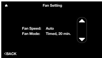
**Fan Mode** – This feature allows you to define the minimum amount of time each hour that the system fan will run. The default is continuous and the fan will run in between heating and cooling calls constantly. You can adjust the minimum fan runtime between 10 and 40 minutes per hour. The fan runtime applies during any mode selected except when the system is turned off.
