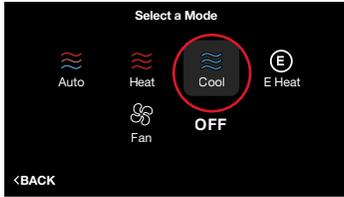
**Cool** – Turns on cooling when the current temperature rises above your set point temperature. When there is an active call for cooling, the words 'Cooling To' will appear above the cooling set point.
