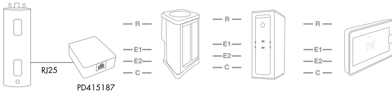
Example of Smart Thermostat connection with HVAC and Water Heater unit. Please note this is an example only, and the ordering network can change as long as it is daisy chained.
