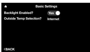
**Outside Temp Selection** – The selection determines where the outside temperature that is displayed on the home screen is pulled from. Choose between Internet and Equipment.
