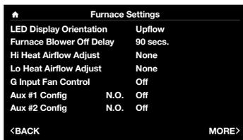
**LED Display Orientation** – Flips the furnace’s LED diagnostic display so it is readable in the upflow or downflow position.
