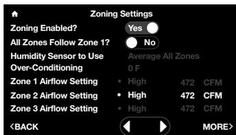
On the Zoning Settings menu, set Zoning Enabled to 'Yes' to display applicable zone settings. From this screen you can select which zone you want to use to track relative humidity, customize airflow noise limits and name zones.
