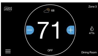
*If you have an **EcoNet Zoning System** and the EcoNet Zone Control heat set point is set to 50°F (10°C) or the cool set point is set to 92°F (33°C), the Zone Control will default to **Off**.*
