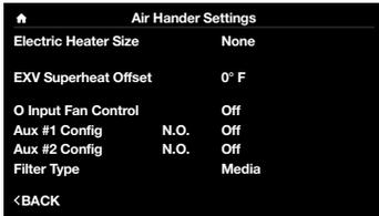
**Electric Heater Size** – If electric strip heaters are installed in the air handler you will need to select the appropriate size.
