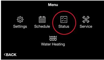
Tapping Menu > Status will display the connected communicating equipment, thermostat mode and the equipment operating status.
