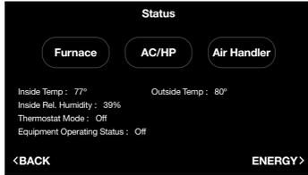
Selecting Furnace, Air Handler or AC/HP on the Status screen will display each piece of equipment's current operating status and historical cycles and run times.
