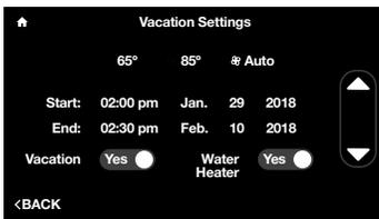
Select each set point and fan speed and then use the up down arrows to set to your desired vacation conditions. We recommend setting the fan speed to Auto.
