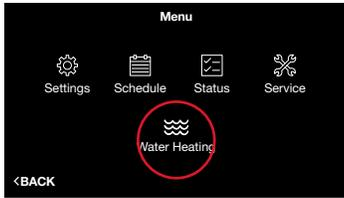
If an EcoNet Enabled water heater is connected to the system, you will see a Water Heating icon under Menu.
