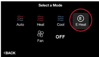
**E-Heat (Heat Pump Systems Only)** – The emergency heat option is a manual setting, not an automatic function initiated by the heat pump thermostat. The purpose of the emergency heat setting is to bring the backup heat source online immediately to deliver 100% of the home's heating demand while simultaneously locking out the heat pump.
