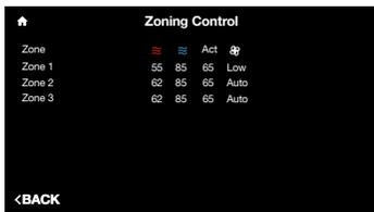
When a zoning system is set up you can view and change the set points and fan speed for zones 2-6 using the zone 1 smart thermostat.
