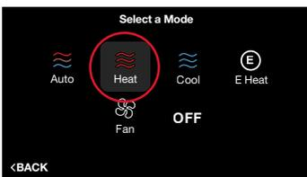
**Heat** – Turns on heating when the current temperature drops below your set point temperature. When there is an active call for heating, the words 'Heating To' will appear above the heating set point.
